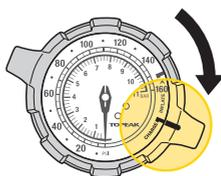
Engage the valve and turn to **CHARGE** mode.
