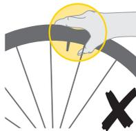
DO NOT squeeze tire when engaging pump head as it may separate tire and rim and prevent a good seal when inflating.
