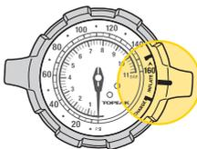
DO NOT turn Mode Selector to mid-point between modes. The pump will not function properly and the gauge will display \*0 psi/ 0 bar.
