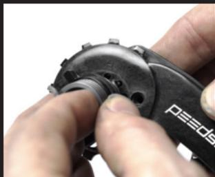
10. Mount the factory spring and plastic spacer onto the face of the OSPW X System. Make sure that the plastic cover is placed exactly the same way on the OSPW X System as on the Shimano assembly. The flat face should sit against the OSPW X System.
