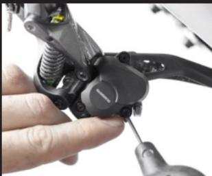
4. Remove the 3 screws on the clutch cover with a 2mm Allen Key. Please note the rubber gasket that sits between the clutch cover and derailleur body. Carefully set the cover, gasket and screws aside as they will be reinstalled.
