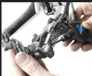
6. Once the cage is free, be careful not to drop the pulley spring and/or plastic spacer.
