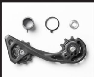
7. Remove the spring and plastic spacer from the Shimano cage and set it aside. The end of the spring is hooked to lock into the pulley cage, you may need to wiggle the spring to release the hook from the cage. Remove and keep the silver washer for use on the OSPW X system.
