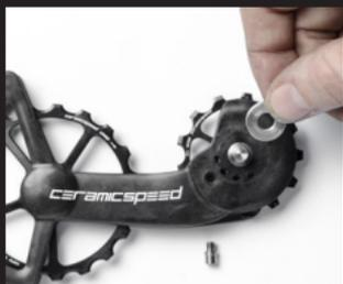
9. Install the flat silver washer from the stock cage onto the OSPW X body, over the threaded post.
