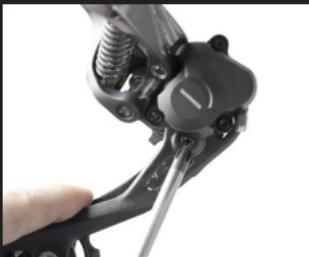
3. Next, shift the derailleur up, past the cable routing/motor point. Rotate the pulley cage (A) downward, locate and remove the Philips head pulley cage stop screw (B). Carefully allow the pulley cage spring to unwind, releasing the spring tension. Your derailleur cage will appear to be upside down.
