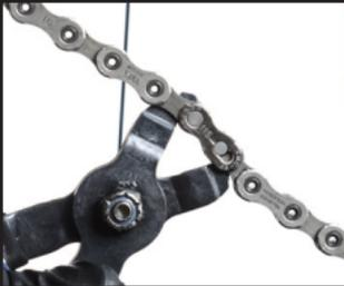
2. Remove your chain by using the proper chain tool. When completing the installation of the OSPW System you will need to start with a new, uncut chain.
