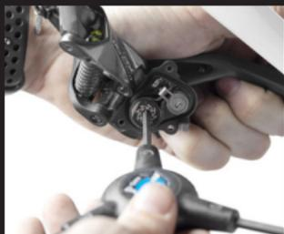
5. Hold the pulley cage and loosen the main mounting screw inside the clutch with a 4mm Allen key to remove the stock cage. Take care that the clutch remains in the original position, flat against the derailleur body.
