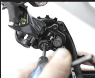
12. Carefully align the female threads of the cage with the male thread in the derailleur body and slowly tighten to avoid cross threading the cage. Hold the OSPW cage still and tighten the original main mounting screw inside the clutch with a 4mm Allen key to 5.5 Nm. Take care that the clutch remains in the original position during the tightening.
