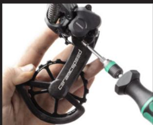
14. Rotate the cage counter-clockwise (up first and then backwards) to increase the spring tension. Once rotated far enough around, mount the CeramicSpeed stop screw with a 2,5mm Allen key. Tighten to 0.3 Nm.
