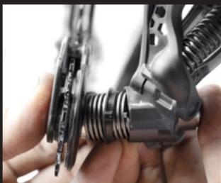
11. Pull the derailleur body back, and position the OSPW X cage facing forward. With the spring and plastic cover on the OSPW X, align the tension spring and plastic cover into the square shaped slot of the derailleur body and insert it until it sits flush. Pivot the system back and forth to ensure smooth movement and spring engagement. The clutch mechanism may be pushed out slightly during this.
