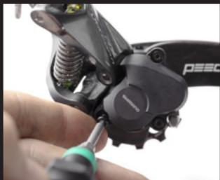
13. Put on the clutch cover (be aware of the gasket) and mount the 3 screws on the clutch cover with a 2mm Allen Key to 0.8 Nm.
