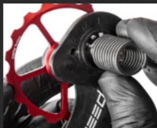
7. Note the three spring tension settings on the OSPW cage: H (high), M (medium) and L (low). The L tension setting will reduce both chain tension and friction, but will also result in slightly compromised shifting performance. The H tension setting provides the best in shifting performance, yet it will increase friction performance slightly over the L and the M tension settings.
