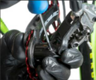
10. Install the original silver mounting screw using the Phillips screwdriver. Once a few threads are secured the OSPW cage should be secured in place. With the cage secured on the silver mounting screw, thread the screw in until tight. This is approximately 0,2 Nm.
