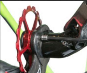
11. Pull the cage up and backwards (counter clockwise) to add spring tension. While holding the OSPW cage down against the spring tension, locate the rotation stop screw mounting hole. Mount the rotation stop screw (7) and tighten it to 0,3 Nm.
