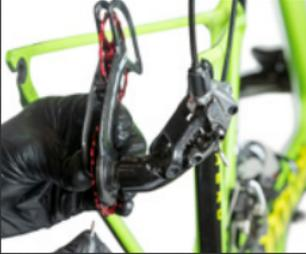
9. Insert the OSPW cage pivot (6) and tension spring into the derailleur body. The cage should sit flush against the derailleur body. Test the fit by rotating the OSPW cage counter clockwise and back forward. Using the original mounting silver screw (see step 3), press the screw into the derailleur body until you reach the threads. The OSPW cage is not secured in place yet.
