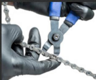
2. Using the proper chain tool, remove your chain. When completing the installation of the OSPW System you will need to use a new, uncut chain. Note: it is not recommended to add links to a previously ridden chain.
