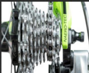
1. Begin with your bike mounted in a stand. Shift to the lowest (smallest) cog and remove the rear wheel. Shift the derailleur to the largest (most open) gear setting for easier access.
