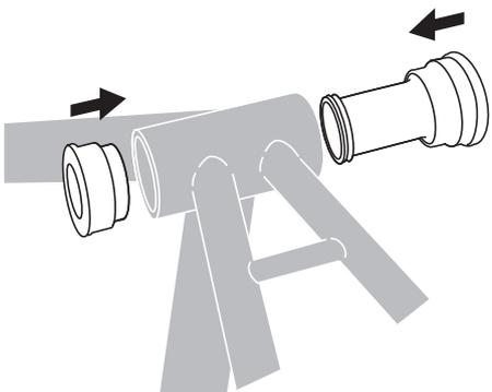
Insert the bottom bracket into the bottom bracket shell.
