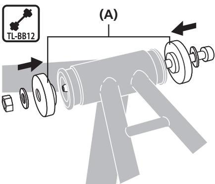
Insert the Shimano original tool into the bottom bracket.
