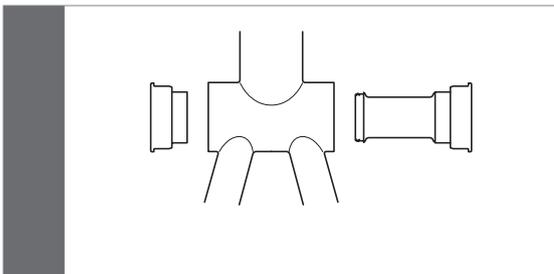
Use for a bottom bracket shell width of 86.5 mm.
