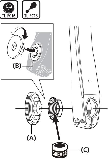
Use the Shimano original tool to tighten the cap.
