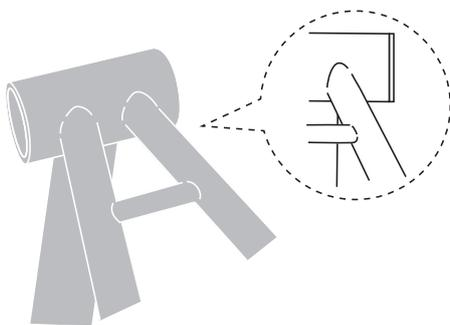
Check to confirm that there is no gap between the bottom bracket and the bottom bracket shell.
