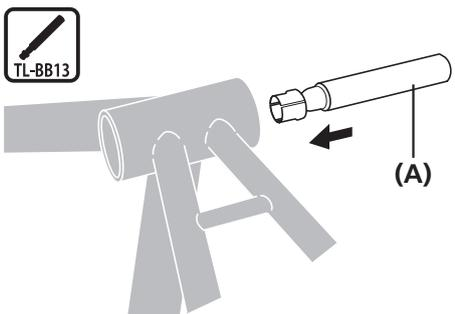
Insert the Shimano original tool into the bottom bracket.
