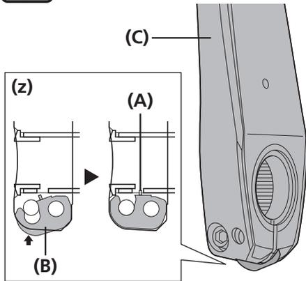
Push in the stopper plate and check that the plate pin is securely in place, and then tighten the bolt of the left crank arm.
