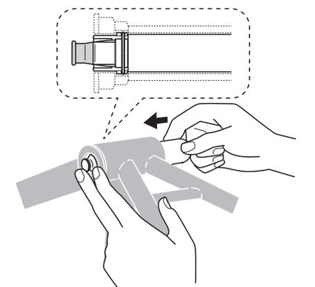
As shown in the illustration, hold down the flap with your fingers and push it in from the opposite side. (When pushed in, the flap opens.)
