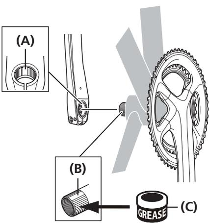
Set the wide groove area of the left crank arm into the axle of the right crank arm unit where the groove is wide.
