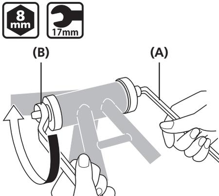
Press fit the bottom bracket by tightening with a spanner while making sure that the contact surface of the bottom bracket stays parallel to the contact surface of the bottom bracket shell.
