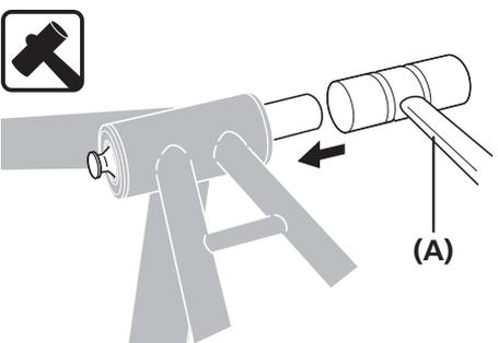
Tap the Shimano original tool with a plastic mallet until the end of the bottom bracket is ejected.
