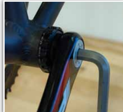
9. Install left crank arm, tighten crank to manufacturer specifications, approximately 48-54 Nm. Add spacers as necessary to take up any play, remove spacers as necessary if binding occurs.
