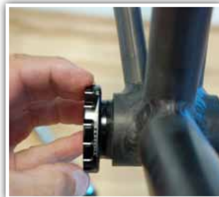
3. Insert drive side cup and center sleeve into frame.
