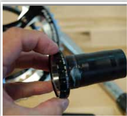
2. Apply a thin layer of grease to cup.
