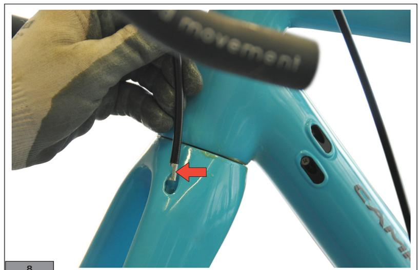
**8)** Assess the correct length of the hose by observing its position in the handlebar area and bearing in mind that the part entering the calliper should measure 11 mm in length from the cut end of the hose (Fig. 9). Once the barb (with the head measuring 4 mm in length) has been inserted, the part of the hose and barb entering the calliper should measure approximately 15 mm.
