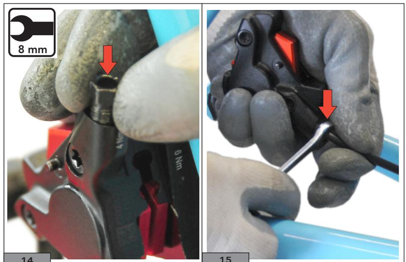
**13)** Once it has been sufficiently tightened, unscrew the nut in order to extract the hose and check that the chamfering on the olive allows the barb to protrude from the olive itself (Fig.16). If this is not the case, you must return to step 7 and cut the end of the hose, otherwise the seal between the hose and barb would not be effective.
