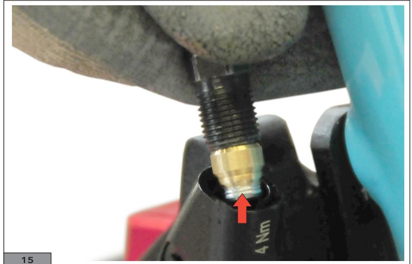
**16)** Insert the hose into the calliper once again, screw on and tighten the nut again to the prescribed torque, taking care not to damage the hose with the tool (Fig. 17).
