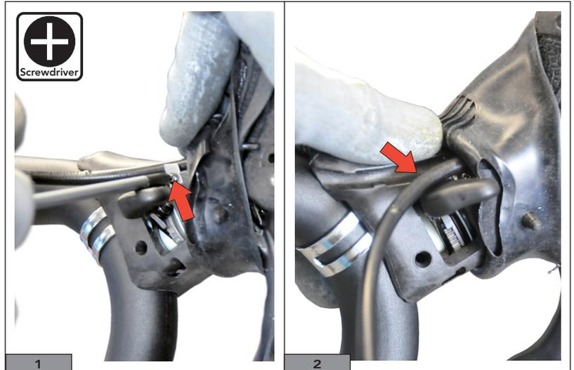
16) Remove the hose from the groove on the command body (Fig. 2).
