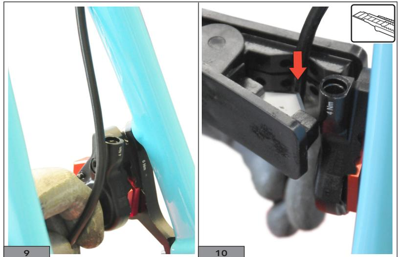
**10)** Insert part of the barb into the hose and push it in using the driver tool (Fig. 11).
