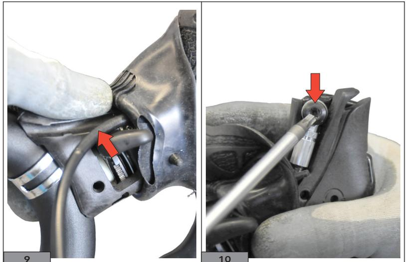
10) Remove the hydraulic hose from beneath the command cover (Fig. 11).
