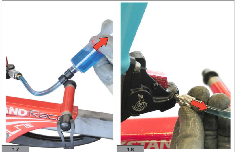
**16)** Remove the syringe from the calliper (Fig.18).
