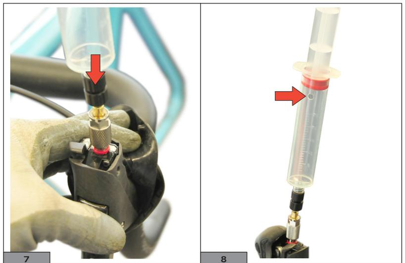
7) Push the plunger of the syringe connected to the calliper (Fig. 9) to expel all the air trapped in the system until the oil exiting from the command bleed valve has filled the syringe by at least 50 %. Ensure that the bottom syringe is not left without oil, so as to prevent air from entering the calliper.
