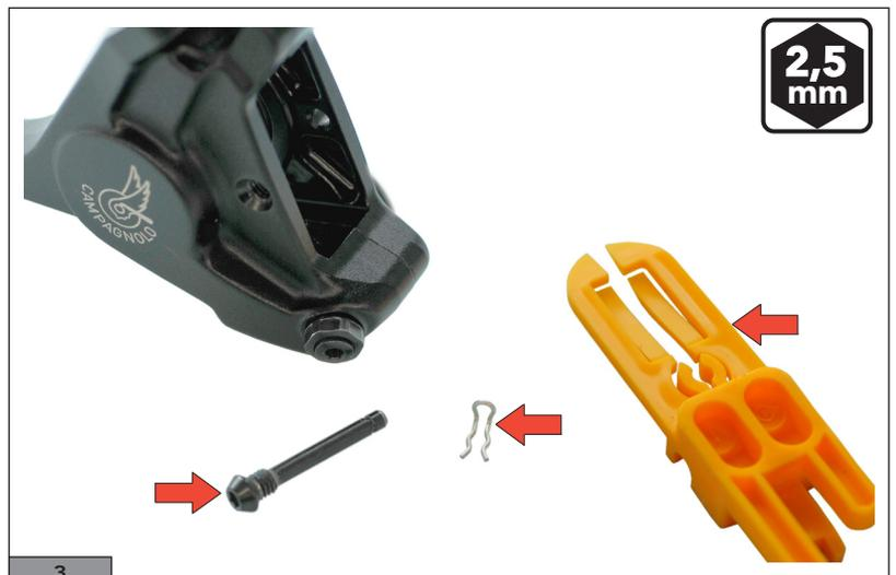
3) Fit the oil level tool (which has a width of 10.5 mm). If necessary, push the pistons back into the calliper using the transportation block (Fig.4).
