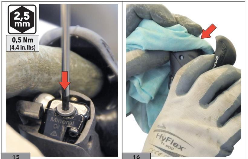
**15)** Remove the oil between the valve and the syringe connection, aspiring with the syringe to prevent any remaining oil underneath the valve screw from leaking once this is in place in its seat (Fig.17).
