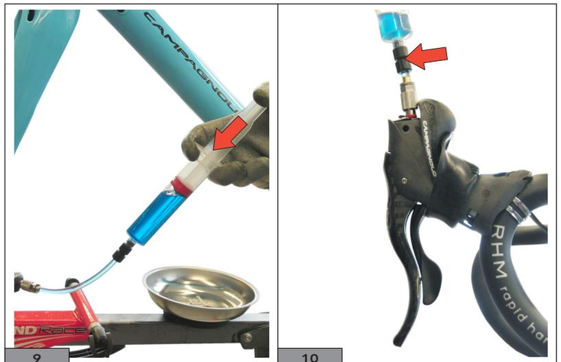
8) Slowly aspirate oil with the syringe connected to the calliper, watching for air bubbles, until the syringe is at least 50% full. Ensure that the top syringe is not left without oil, so as to prevent air from entering the calliper.(Fig.10).
