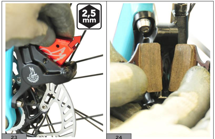
22) Position the pads so that the metal support is in contact with the pistons (Fig. 24).
