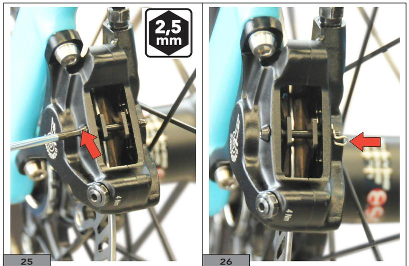
24) Position the securing pin on the pivot (Fig. 26).
