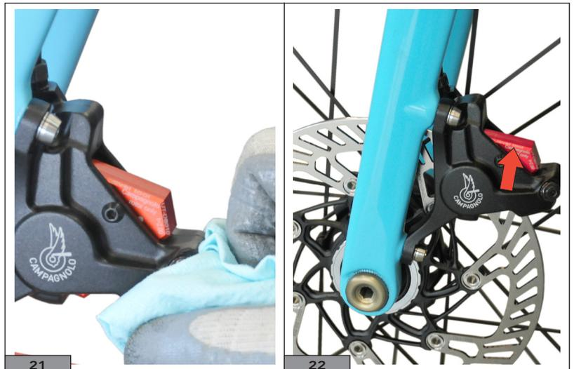
**20)** Refit the wheel and align the calliper with the disc, with the centring tool still in the calliper: this is to provisionally align the calliper with the disc (Fig. 22).
