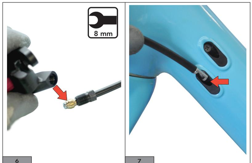
The barb driver on the end of the hose can be used to guide the hose via a rear derailleur hose mounted onto it (Fig.).
