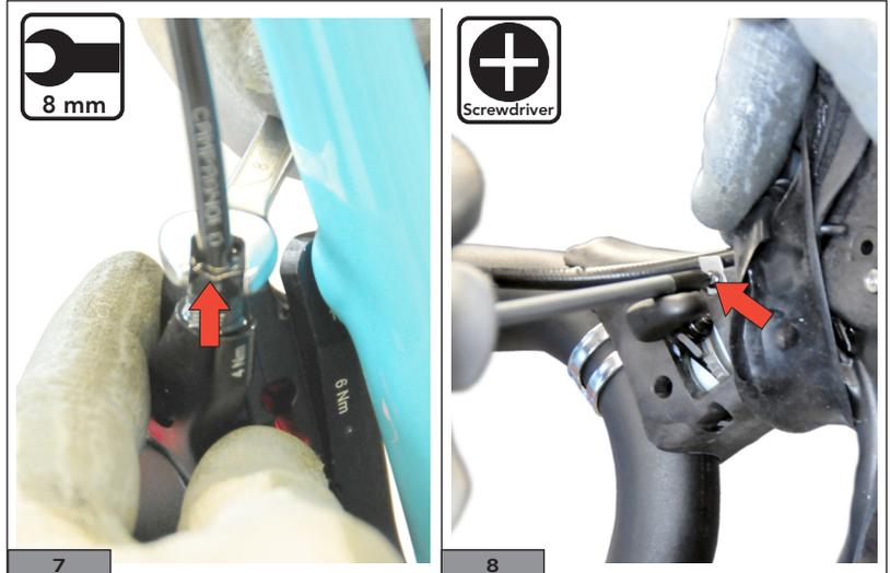
8) Remove the hose from the groove on the command body (Fig. 9).
