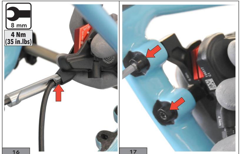
**17)** Temporarily install the calliper onto the left-hand chain stay fitting the two Campagnolo screws following the indications in the table on the right, which ensures that the screws are inserted at least 5 mm into the calliper.
