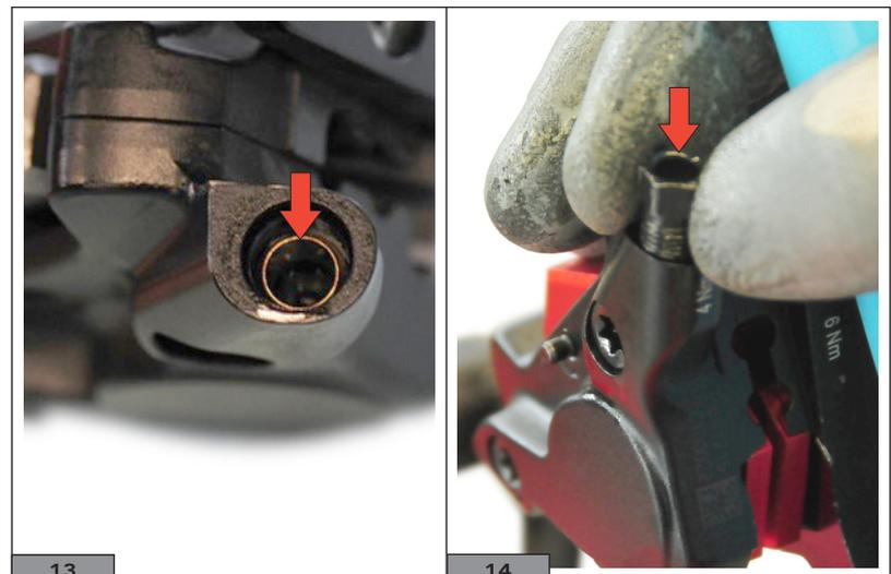
**14)** Insert the hose into the calliper and tighten the nut ensuring that the hose is properly inserted into the calliper (Fig. 15).
