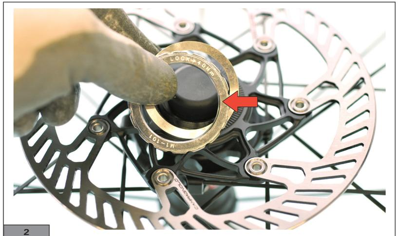
3) Screw on the locknut (Fig.3).
