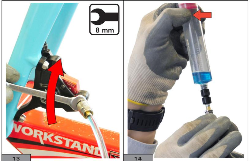
13) Check that there is oil in the screw seat and tighten the bleed screw (Fig.15).
