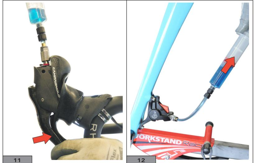
11) When all air has been expelled, ensure that the level of oil in the syringe is above 1 cm approx. and close the bleed valve by turning the key clockwise (Fig.13).
